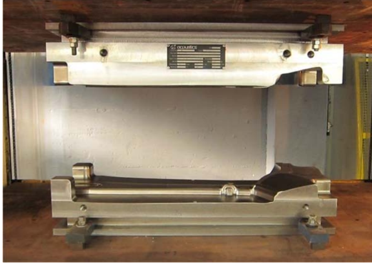
Figure 2. Steel mould properly realized to process Brigit demonstrator
