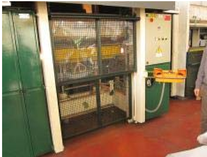
Figure 5. Heating press used for the heating step before the moulding of the component
