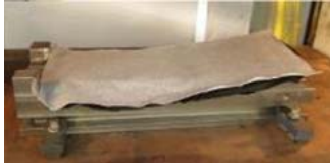
Figure 6. Application of aesthetical TNT on component before the moulding process
