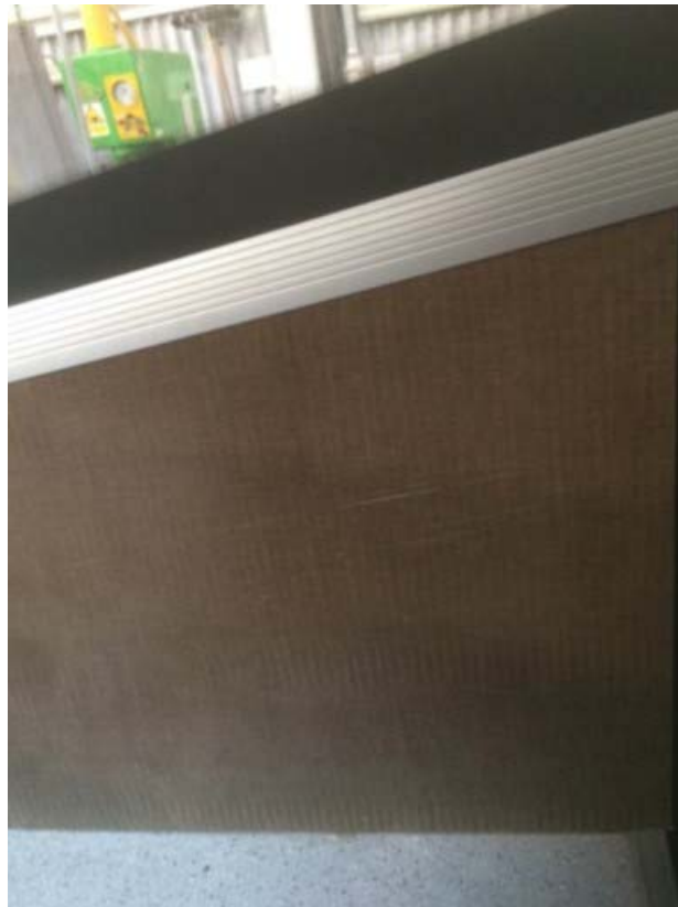
Figure 9. Front pillar cover for truck realised using new developed Brigit material.
