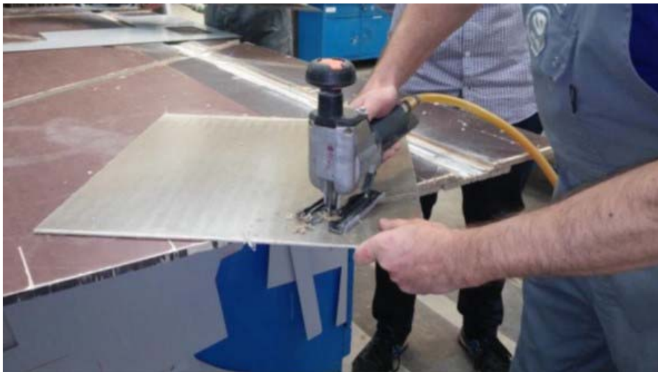
Figure 10. Tooling test – using fretsaw.
