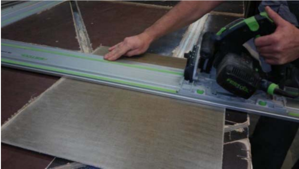
Figure 12. Tooling test – using saw.
