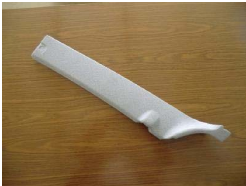
Figure 5. Front pillar cover for truck realised using new developed Brigit material.
