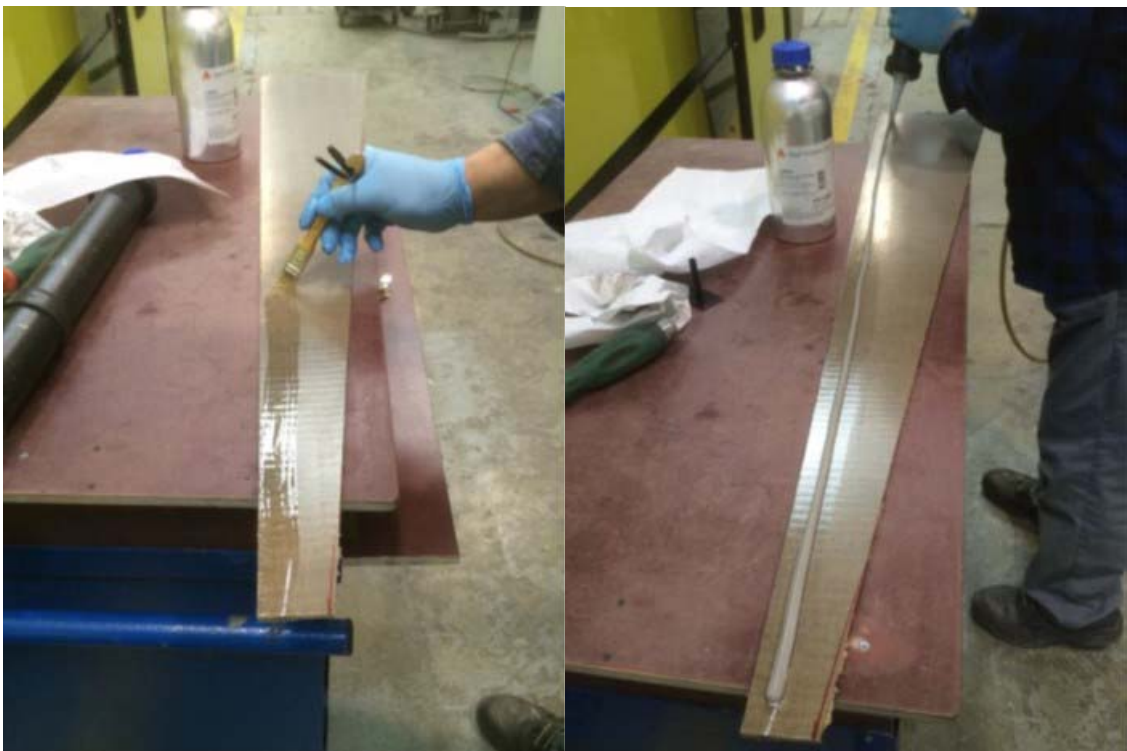
Figure 14. Adhesives tests primer (left) and adhesive (right) application.
