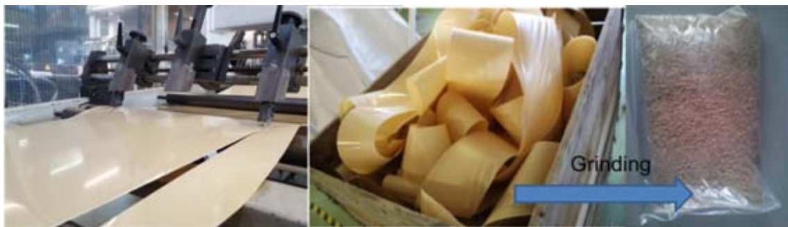
Figure 18. Laminate, trimmed edges of the laminate and scrap.
