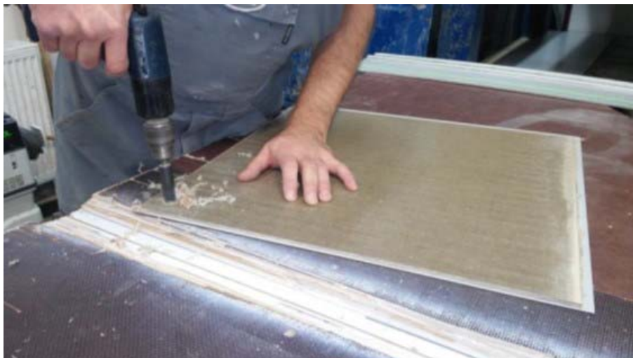
Figure 11. Tooling test – using hole saw.
