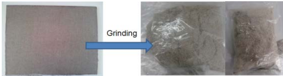
Figure 17. Left: sandwich panel. Right: Ground sandwich panel.
